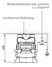
The extinguishing chamber cover is part of the standard scope of delivery for the C360A/150, C360A/300 and C360A/500 series.
