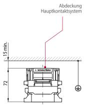
For the C360S/150, C360S/300 and C360S/500 series there is a minimum distance of 15 mm to magnetically active, live or earthed parts.
