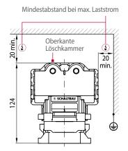
For the C360K/150, C360K/300 and C360K/500 series there is a minimum distance of 20 mm to magnetically active, live or earthed parts.
