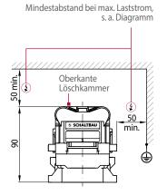
It is permissible to use the C360A/150, C360A/300 and C360A/500 series without arc chamber cover, taking into account additional clearance dimensions.
