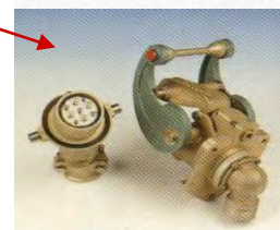
ELECTROPNEUMATIC BRAKE UIC 541-5 Connector
